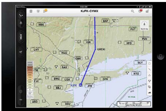
Applications for iPads and other mobile devices save weight and allow pilots to filter information, providing the necessary information at the right time—making navigation more efficient. (Jeppesen image)
