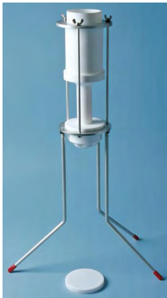
Figure 1: Dekaport Cone Splitter for making replicate water samples. The device, including legs, weighs 8 pounds and is 26.1 inches tall. The splitter without legs is 13.4 inches in height and is constructed entirely of Teflon ® . The legs and supporting frame are anodized aluminum. From top to bottom, the cone splitter consists of a 4-inch diameter upper reservoir, stand pipe to deliver a uniform flow to the splitter cone, splitter cone chamber, and 10 exit ports to which 3/8-inch O.D, Teflon ® tubing can be attached for collecting split samples.
