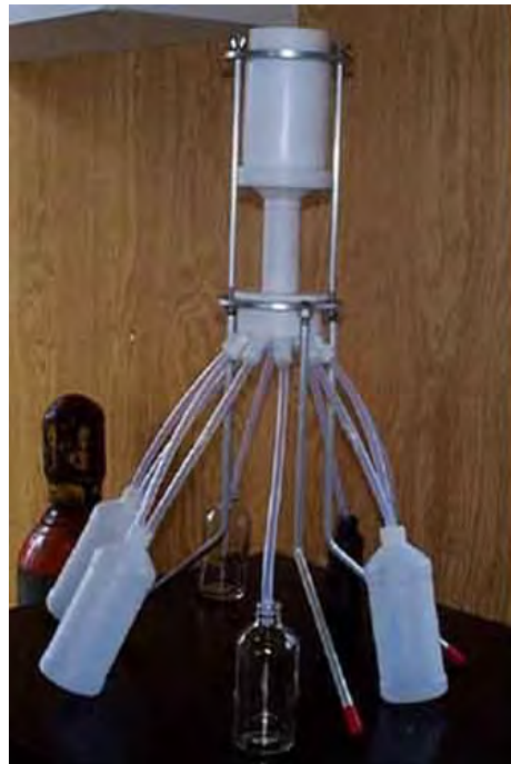
Figure 2: Cone splitter with different kinds of collection containers attached. The three plastic containers are each connected to two outlet ports for collecting larger sample volumes.
