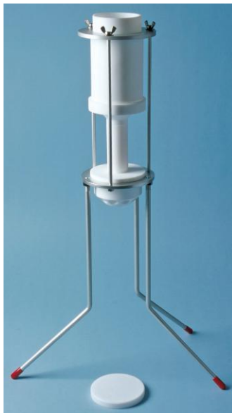
Figure 1: Dekaport Cone Splitter for making replicate water samples. The device, including legs, weighs 8 pounds and is 26.1 inches tall. The splitter without legs is 13.4 inches in height and is constructed entirely of Teflon ® . The legs and supporting frame are anodized aluminum. From top to bottom, the cone splitter consists of a 4-inch diameter upper reservoir, stand pipe to deliver a uniform flow to the splitter cone, splitter cone chamber, and 10 exit ports to which 3/8-inch O.D, Teflon ® tubing can be attached for collecting split samples.
