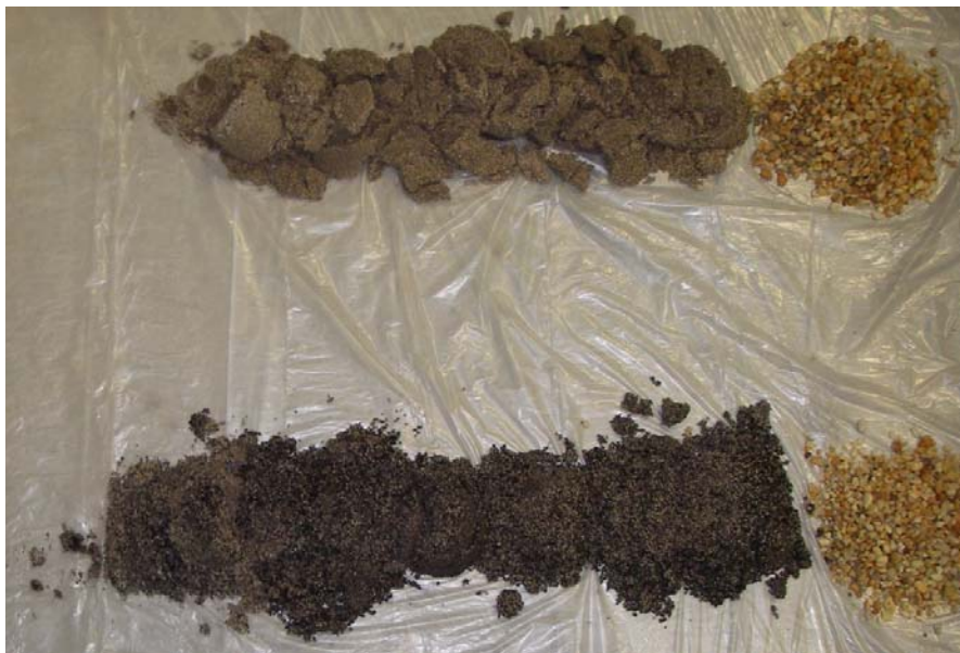
Figure 3-11. Soil Media after Removal from Columns Prior to Soil Sample Collection. Upper layers of the columns are to the left side of the picture.
