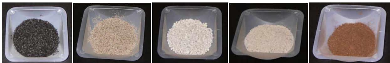
Figure 3-1. Media (from left to right): GAC, Rhyolite Sand, Site Zeolite, Surface Modified Zeolite, Sphagnum Peat Moss
