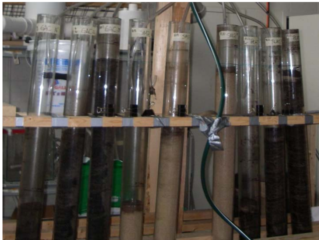
Figure 3-12. Media Depth Test Column Setup (14-inch to 38-inch columns per media from left to right)
