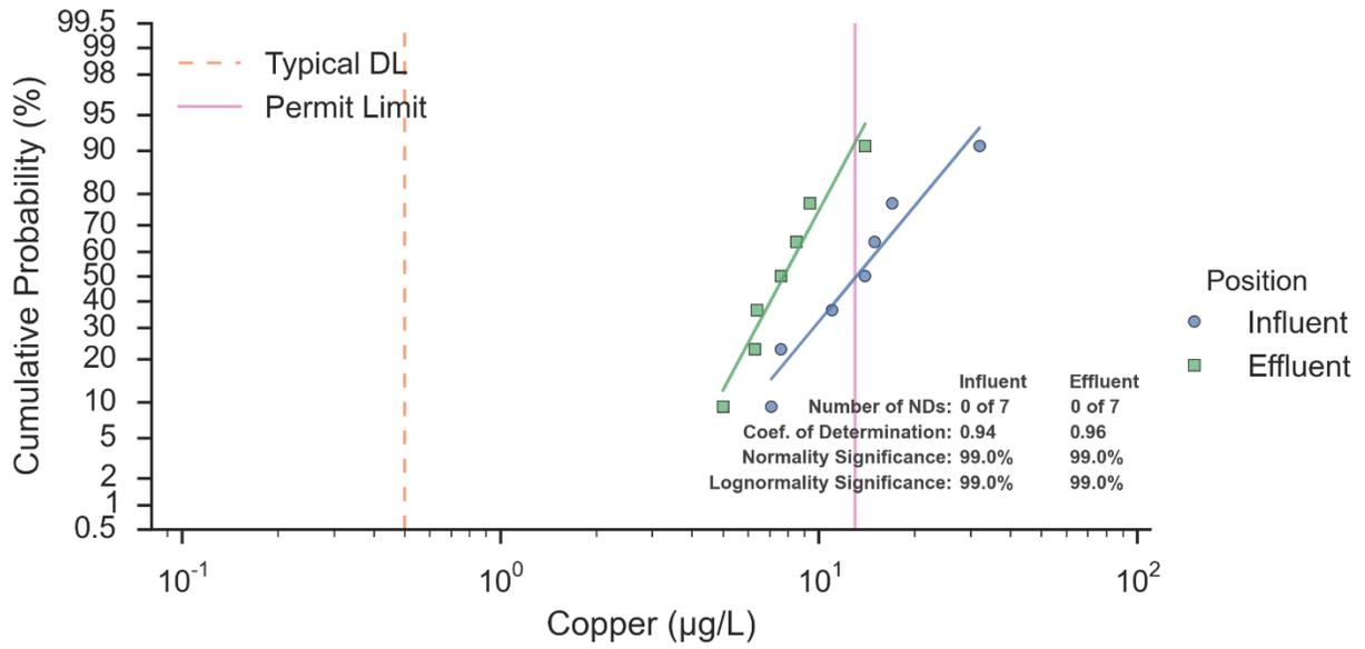
**Figure 58. Probability Plot of Copper at Lower Lot Biofilter**
