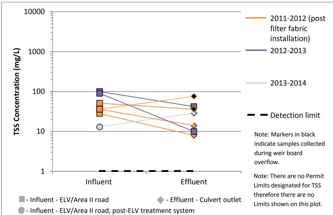
**Figure 2. TSS at CM-1, post filter fabric installation**
