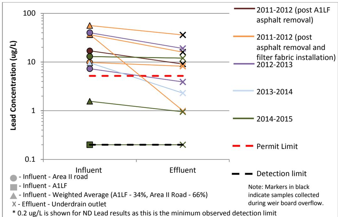
**Figure 25. Lead at CM-9, post improvements (removal of A1LF asphalt and addition of CM weir board filter fabric)**
