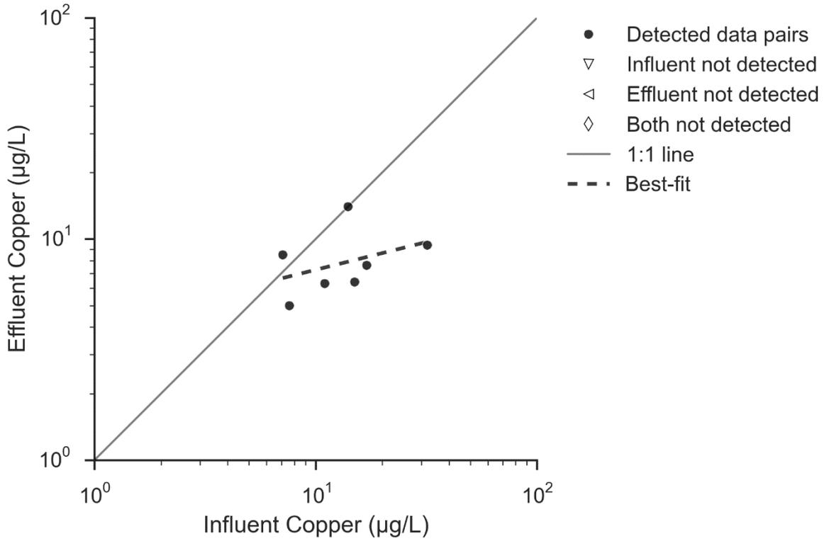
**Figure 46. Paired Copper Concentrations at Lower Lot Biofilter**
