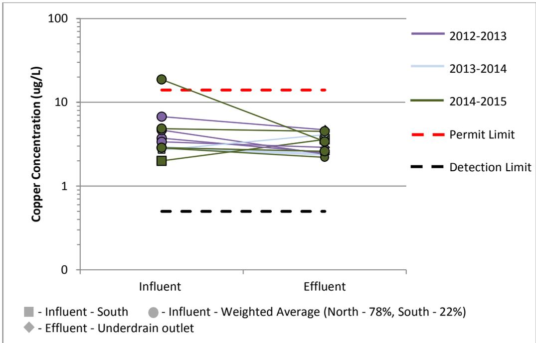
**Figure 35. Copper at B-1 Media Filter (CM), post curb cuts**
