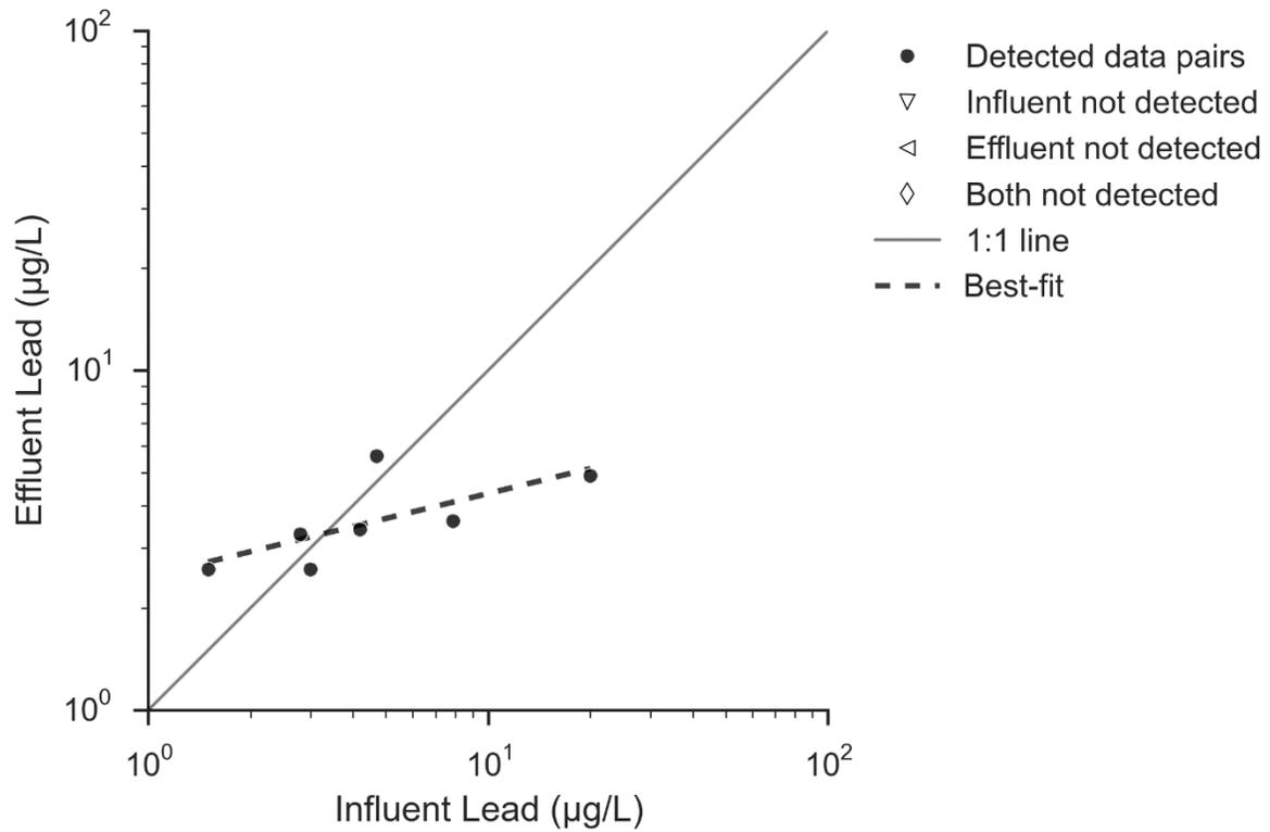
**Figure 45. Paired Lead Concentrations at Lower Lot Biofilter**
