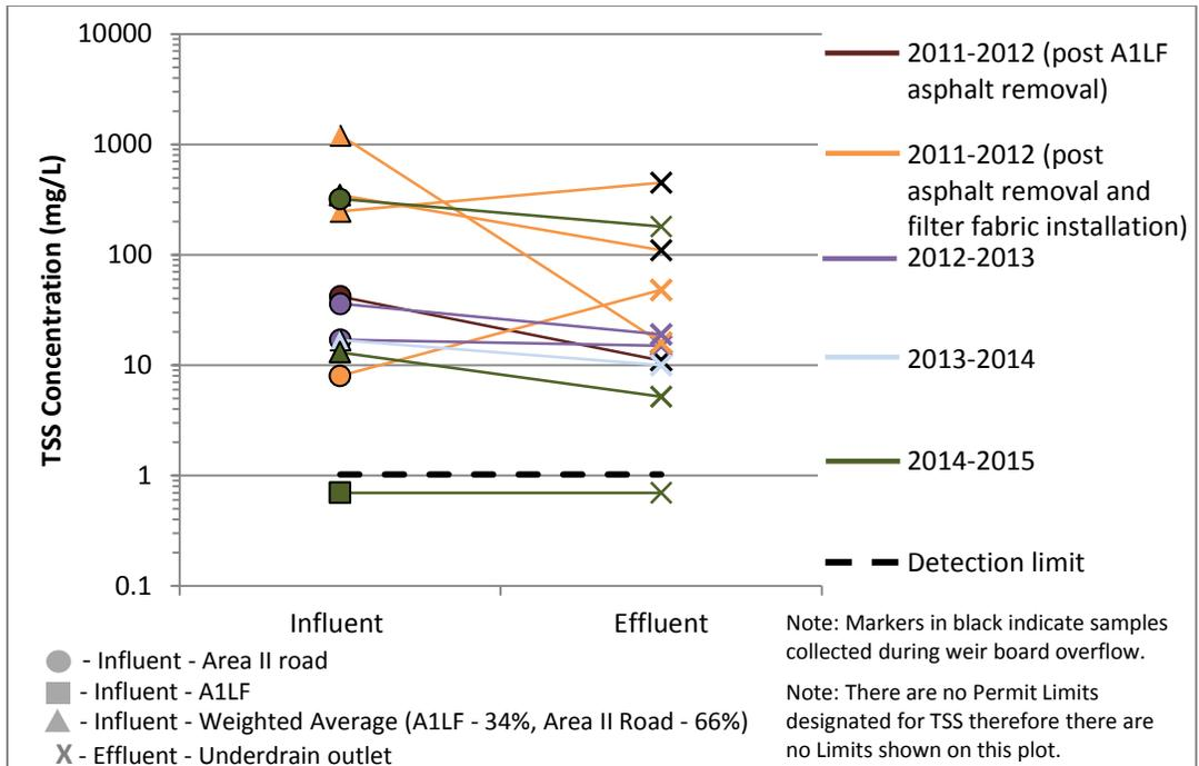
**Figure 5. TSS at CM-9, post improvements (removal of A1LF asphalt and addition of CM weir board filter fabric)**
