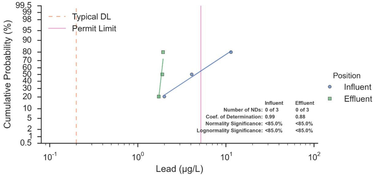
**Figure 61. Probability Plot of Lead at ELV Stormwater Treatment BMP**
