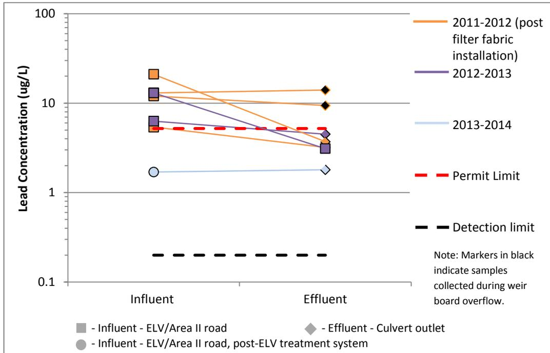
Figure 22. Lead at CM-1, post filter fabric installation
