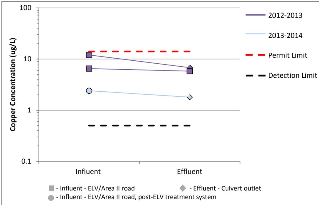
**Figure 31. Copper at CM-1, post filter fabric installation**
