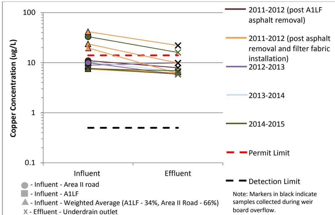
**Figure 33. Copper at CM-9, post improvements (removal of A1LF asphalt and addition of CM weir board filter fabric)**
