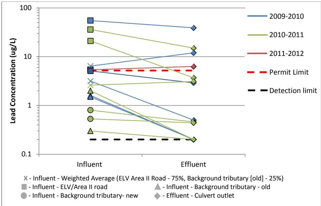
Figure 21. Lead at CM-1, pre filter fabric installation
