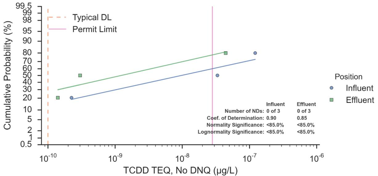
**Figure 60. Probability Plot of Dioxins at ELV Stormwater Treatment BMP**
