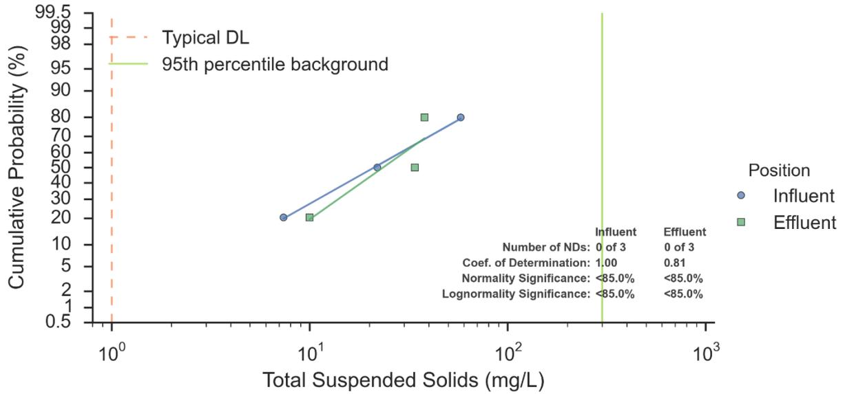
**Figure 59. Probability Plot of TSS at ELV Stormwater Treatment BMP**
