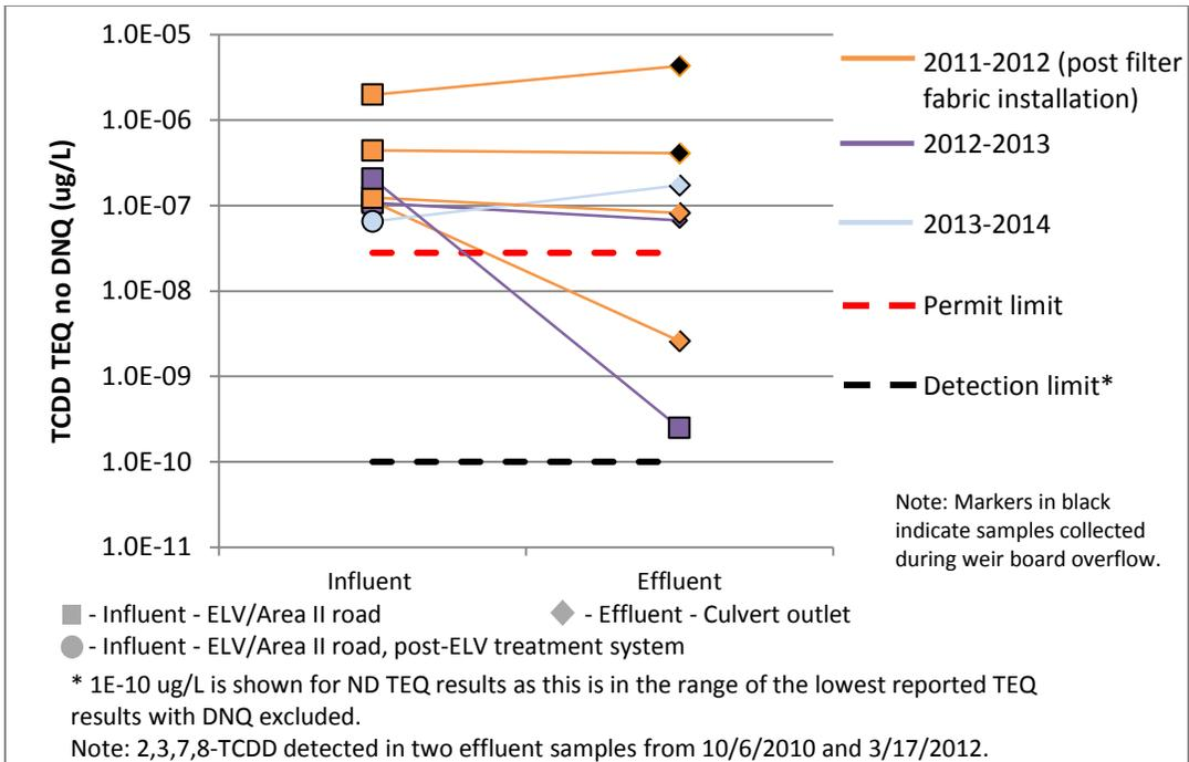
Figure 13. Dioxins at CM-1, post filter fabric installation
