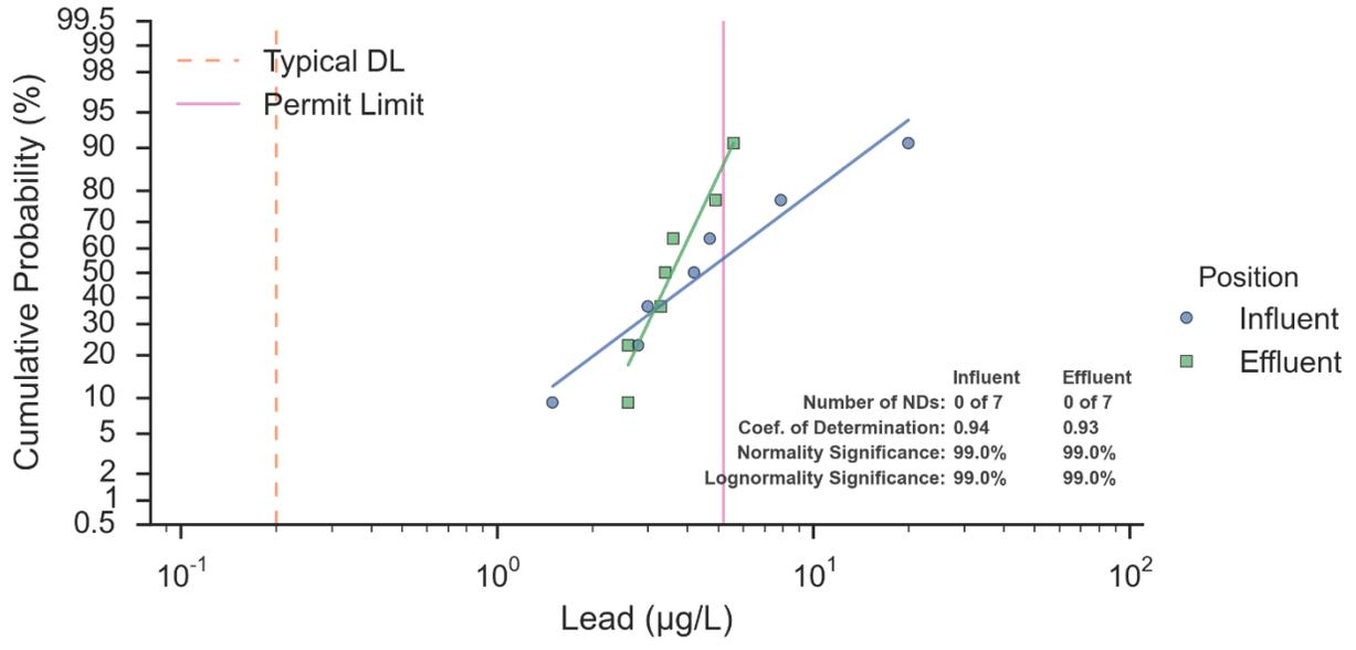
**Figure 57. Probability Plot of Lead at Lower Lot Biofilter**
