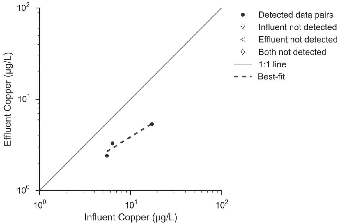
**Figure 50. Paired Copper Concentrations at ELV Stormwater Treatment BMP**
