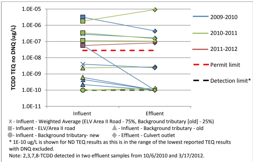
Figure 12. Dioxins at CM-1, pre filter fabric installation
