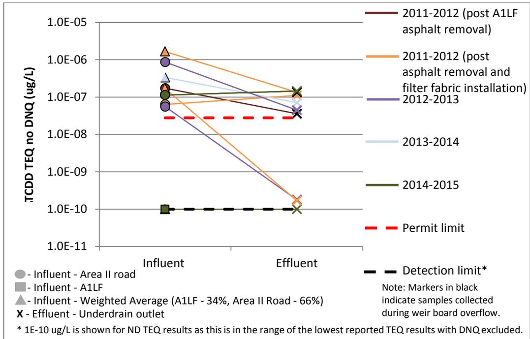
**Figure 15. Dioxins at CM-9, post improvements (removal of A1LF asphalt and addition of CM weir board filter fabric)**
