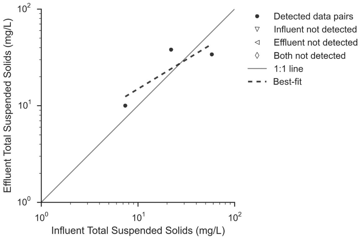
**Figure 47. Paired TSS Concentrations at ELV Stormwater Treatment BMP**
