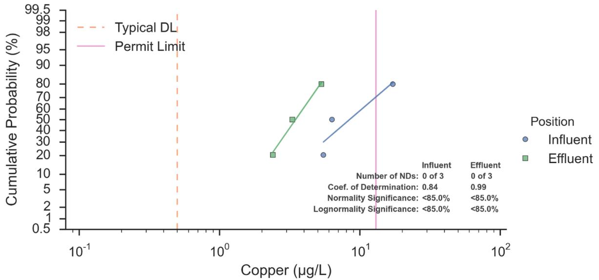
**Figure 62. Probability Plot of Copper at ELV Stormwater Treatment BMP**
