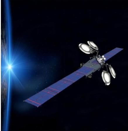
The Boeing 702SP can operate in the S-, X-, C-, Ku, and Ka-band frequencies and, as with all Boeing 702s, is designed to provide 15 or more years of satellite service with additional fuel capacity to enable multiple station changes over the life of the satellite. The 702 family of vehicles is designed to accommodate hosted payloads, such as sensors, UHF, military Ka-band and navigation L-band, resulting in additional flexibility for customers.
