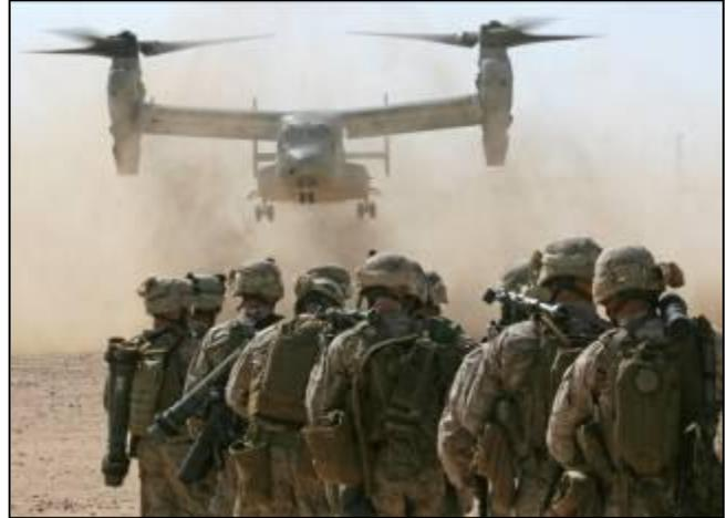
The Osprey can carry 24 combat troops, or up to 20,000 pounds of internal cargo or 15,000 pounds of external cargo, at twice the speed of a helicopter. It features a cross-coupled drive system so either engine can power the rotors if one engine fails. For shipboard compatibility, the rotors fold and the wing rotates to minimize the aircraft's footprint for storage. The V-22 is the only vertical lift platform capable of rapid self-deployment to any theater of operation, worldwide.
