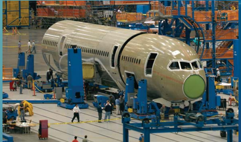
Celebrating the "grand opening" of its 787 final assembly facility in Everett, Wash., Boeing workers assemble the 787's very large composite structures using portable tools rather than traditional monuments and overhead cranes.
