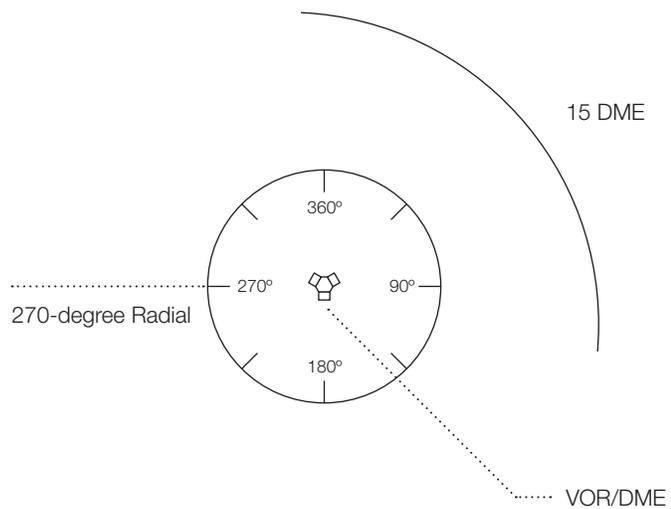
the very-high-frequency omni-directional range (VOR) navigation system and distance measuring equipment (DME). VORs came into wide use in the 1950s and quickly became the preferred navigation radio aid for flying airways and instrument approaches (see fig. 1). VOR and DME provided the framework for a permanent network of low-altitude victor airways (e.g., V-4) and high-altitude jet routes (e.g., J-2), which are still in place today.
