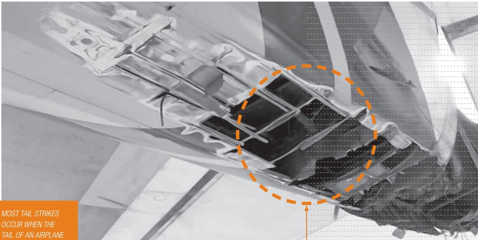
*MOST TAIL STRIKES OCCUR WHEN THE TAIL OF AN AIRPLANE STRIKES THE GROUND DURING LANDING AND ARE PREVENTABLE.*
