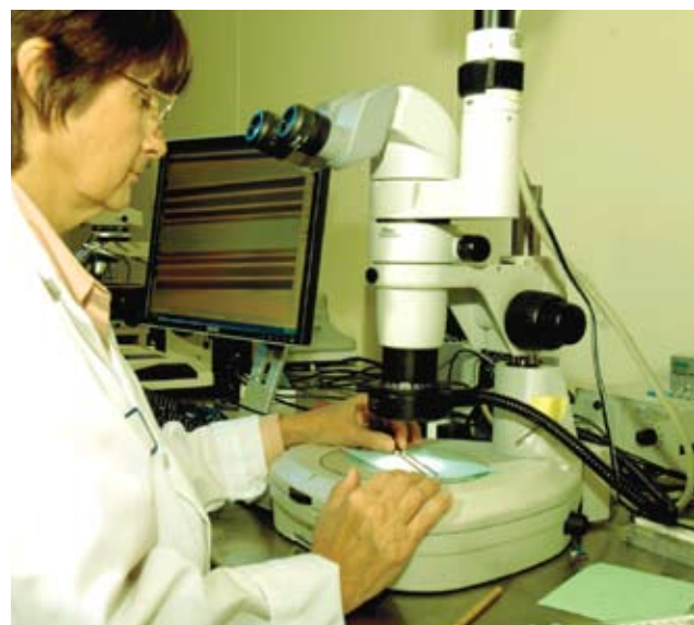
Jean Ray, an Associate Technical Fellow in Fuels and Lubrication Technology for Commercial Airplanes, examines test specimens after exposure to a candidate biofuel. Ray noted that biofuels must be chemically compatible with today's aviation infrastructure. JIM ANDERSON/BOEING
