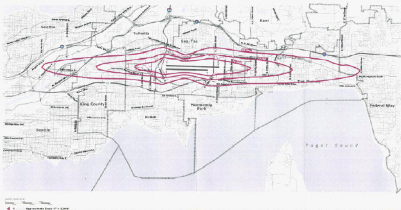
Figure C13 Existing (1998) DNL Noise Contour (Close In View)
