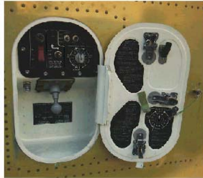
Cargo door/handling system control panel
