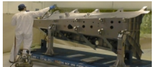
A sol-gel prepaint process was implemented on the F-22 titanium forward boom
