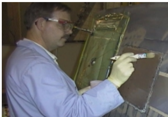
Demonstration of the sol-gel prebond process on a composite patch repair of fatigue cracks on a B-52 fuselage component
