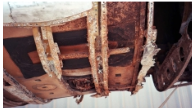
Corrosion on a non-flight-worthy F-86 aircraft fuselage built in the late 40's
