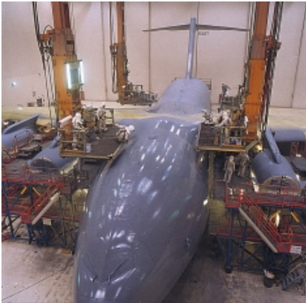
A layer of advanced-performance coating developed by Phantom Works is applied to a C-17 Globemaster III.
