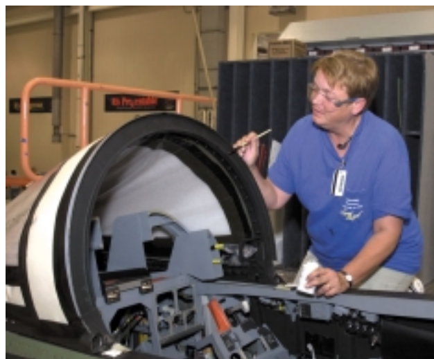
Annette Hammett touches up a Super Hornet cockpit assembly with the new room-temperature paint.
