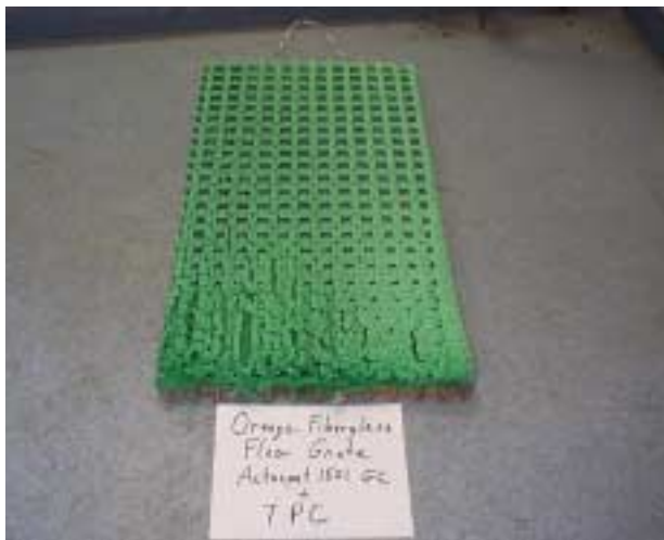
Figure 1 - Before caked coating removal
