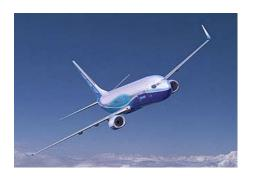
Boeing is driving environmentally progressive technologies into its products and services. Pictured here is a Next-Generation 737-900ER with Blended Winglets, wing tip extensions that lower fuel use, emissions and noise.
