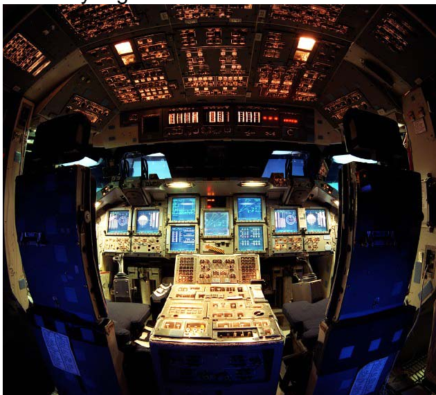
This "fish-eye" view illustrates Multifunction Electronic Display Subsystem (MEDS), otherwise known as "glass cockpit." It represents a number of important modifications that have been accomplished on the Orbiter's flight deck.
