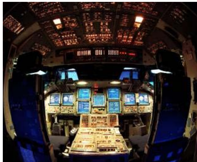
This "fish-eye" view illustrates Multifunction Electronic Display Subsystem (MEDS), otherwise known as "glass cockpit." It represents a number of important modifications that have been accomplished on the Orbiter's flight deck.
