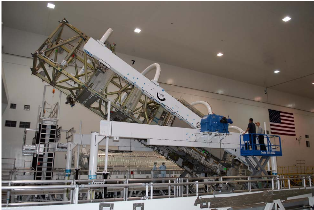
In the Space Station Processing Facility at NASA's Kennedy Space Center, Boeing workers stand ready as the starboard integrated truss, known as S6, is rotated in order to remove and replace lower deck batteries.
