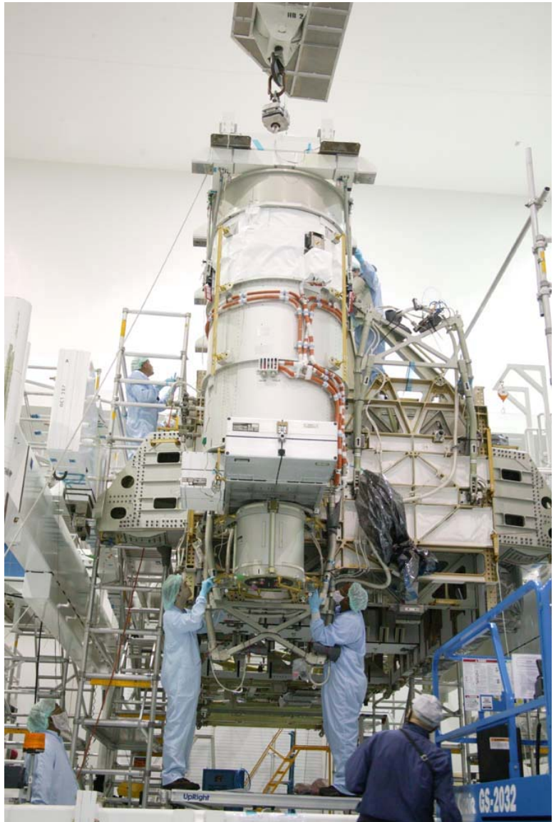
After new batteries were installed on the Starboard 6 lower deck Integrated Equipment Assembly, the Solar Array Wing was reinstalled. Boeing engineer Sam Amundsen is shown on the left of mast canister while Elijah Walker technician is on the right. (Indyne photo by Melanie Gurnavage)
