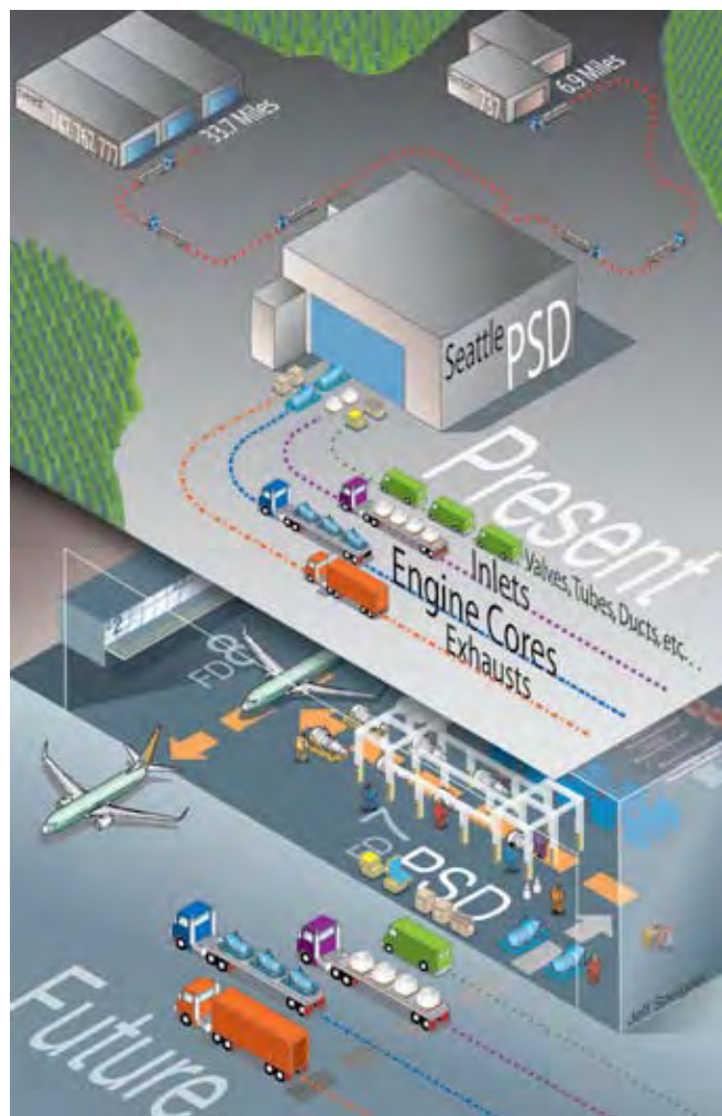
Reduced transportation requirements, improved process flow, and line-of-sight process alignment are among many benefits Commercial Airplanes expects when engine and strut buildup collocates with final assembly in Renton and Everett, Wash.
