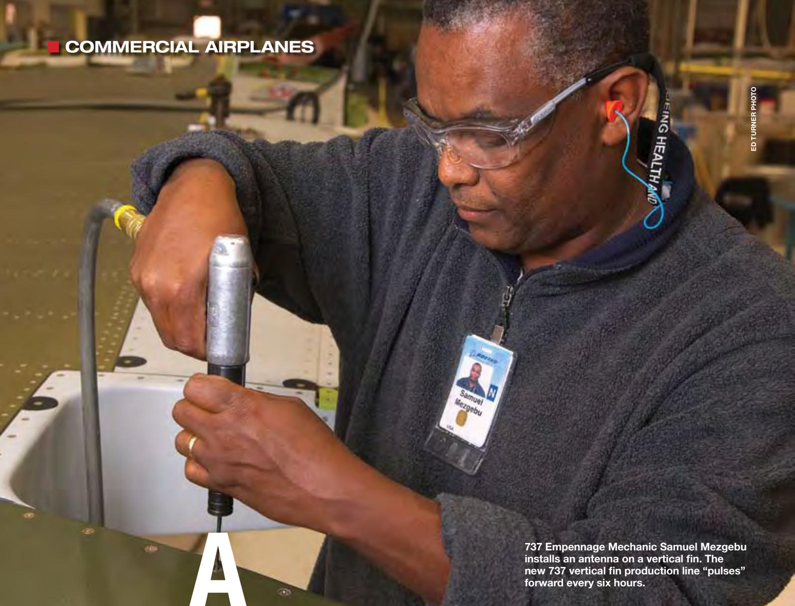
737 Empennage Mechanic Samuel Mezgebu installs an antenna on a vertical fin. The new 737 vertical fin production line “pulses” forward every six hours.
