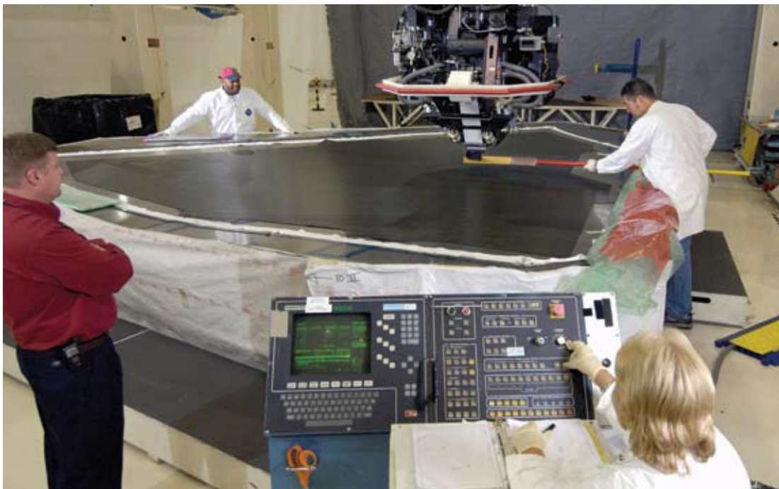
At the Developmental Center in Seattle, operator Arnaldo Rivera (background, right) works with a robotic contour-tape-layup machine to sculpt an F-22 Raptor wing skin into existence. Once operator Pam Parker (foreground) has programmed the CTLM, the machine applies small segments of graphite-composite fabric, laminating them to varying thicknesses for greater flexibility over contoured areas or added strength at stress points. Quality Assurance inspector Anthony Jackson (background, left) and manager Joe Habersetzer keep an eye on the proceedings.
