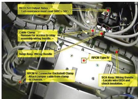
**In this single frame from an augmented reality session, graphic additions are positioned relative to features in a scene. As the viewpoint changes, the graphics change positions as if attached to the features. Boeing hopes to create an augmented reality demonstration project on the International Space Station.**
