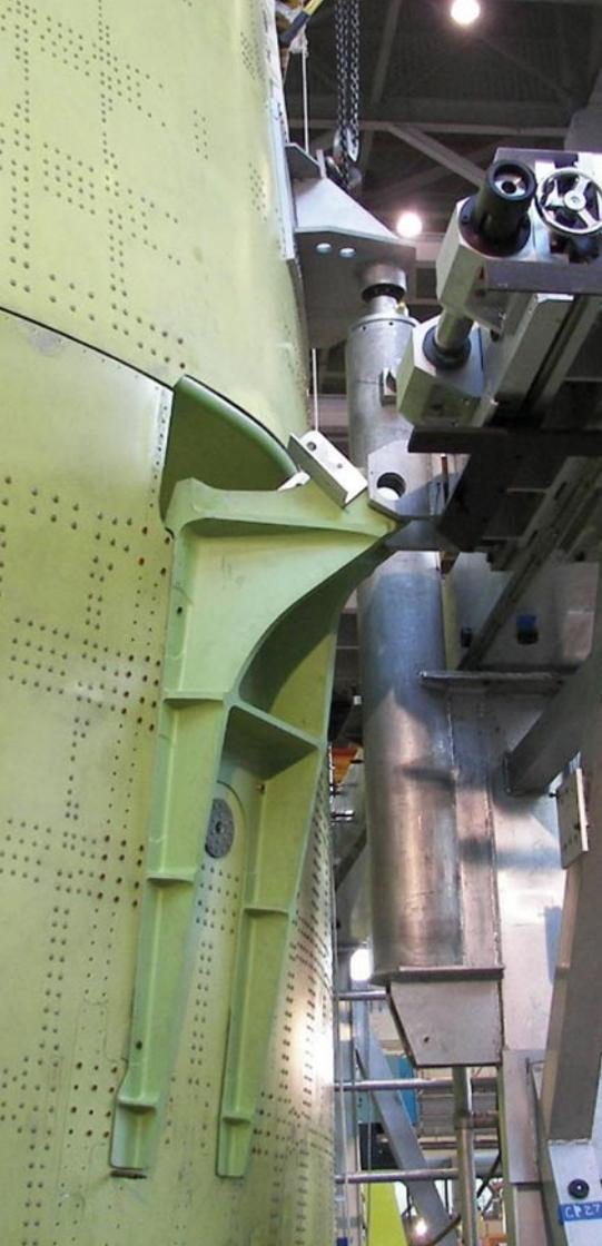
**Boeing Auburn Tooling Services produced the main hinges (above) for the 747 Large Cargo Freighter's tail section. The facility thrives on complex work such as this, said Jeff Krueger, Auburn Tooling Services manager.**
