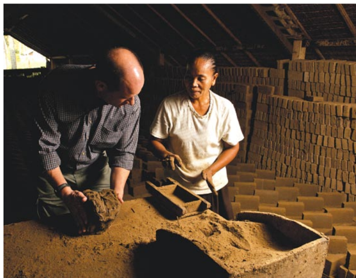
Boeing's Bob Seipel tries his hand at brick making in Lam Ujong, while a worker in the factory looks on. She makes up to 1,300 bricks each day. The factory is actually a small group of modest buildings consisting of a kiln and two thatched-roof open-air structures where the bricks are made and dried.
