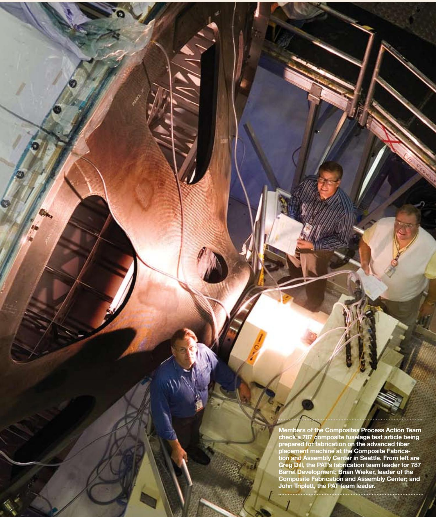
Members of the Composites Process Action Team check a 787 composite fuselage test article being prepared for fabrication on the advanced fiber placement machine at the Composite Fabrication and Assembly Center in Seattle. From left are Greg Dill, the PAT's fabrication team leader for 787 Barrel Development; Brian Wieker, leader of the Composite Fabrication and Assembly Center; and John Triplett, the PAT team leader.
