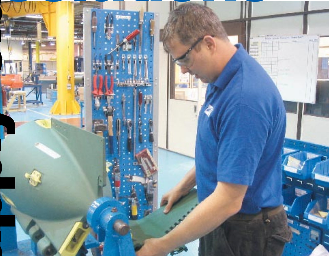
Andy Kershaw of MB Aerospace attaches fins to the aft body of a Harpoon capsule. Following Boeing-facilitated accelerated improvement workshops, MB Aerospace was able to improve the efficiency of this assembly process. MB AEROSPACE PHOTO
