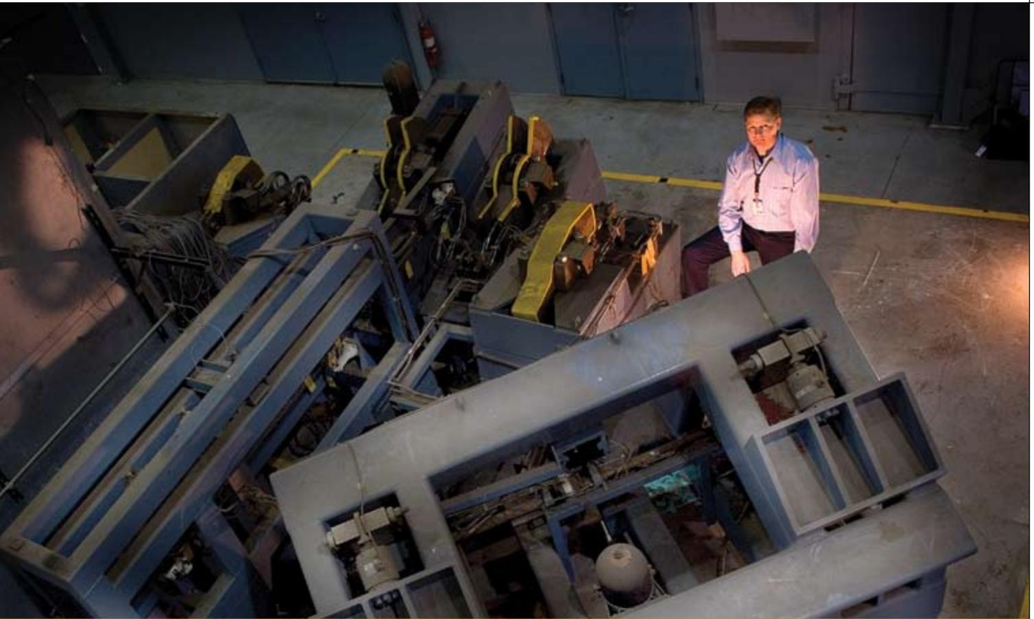
**An unused legacy of the past. Bruce McIlroy, Test and Evaluations Operations manager in St. Louis, is pictured with the A-12 “iron bird,” a massive fixture used to test the hydraulics of the cancelled U.S. Navy aircraft and now no longer needed.**
