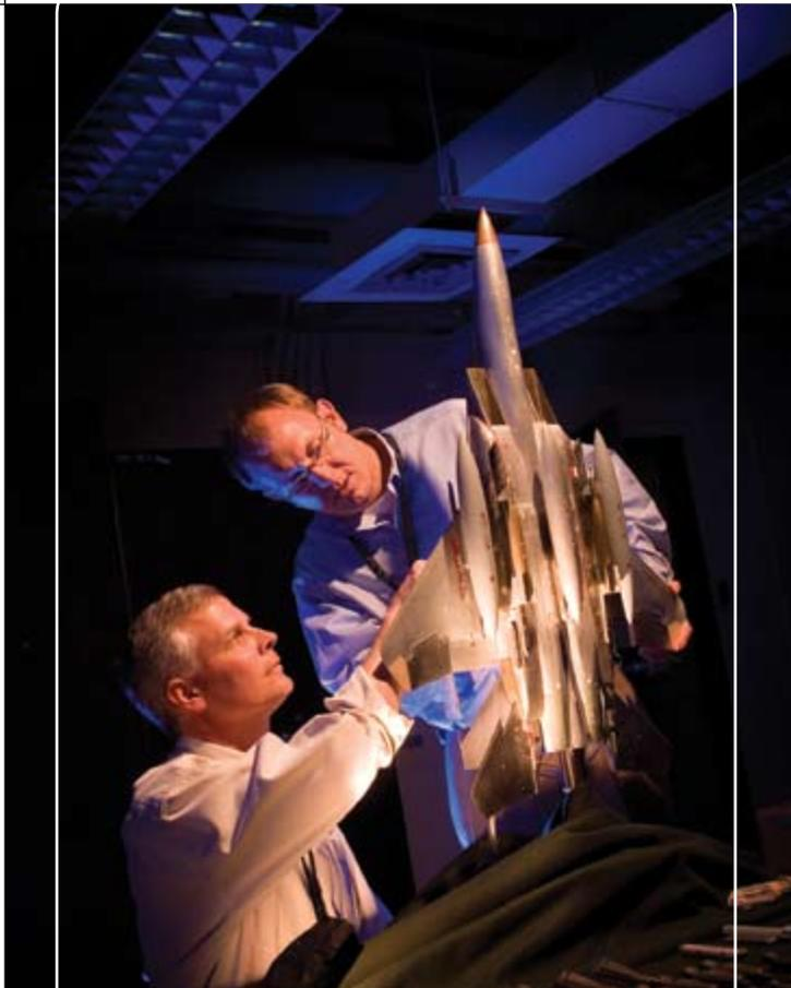
Some test facilities have a bright future. Bob Hilker, manager of Aerodynamics Laboratories in St. Louis (left), and Bill Schane look at a wind tunnel test model of a fully loaded F-15. The model is used in the Polysonic Wind Tunnel in St. Louis, which will continue to be an important test facility for the enterprise.
