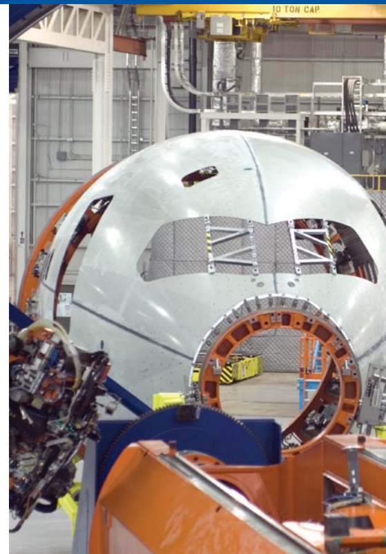
The Spirit AeroSystems 787 factory in Wichita, Kan., is busy building noses for 787s. The plant has approximately seven nose sections in work for the program at any given time.
