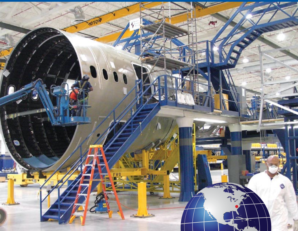
Workers at Vought's South Carolina 787 factory prepare to join their first two barrel sections.
