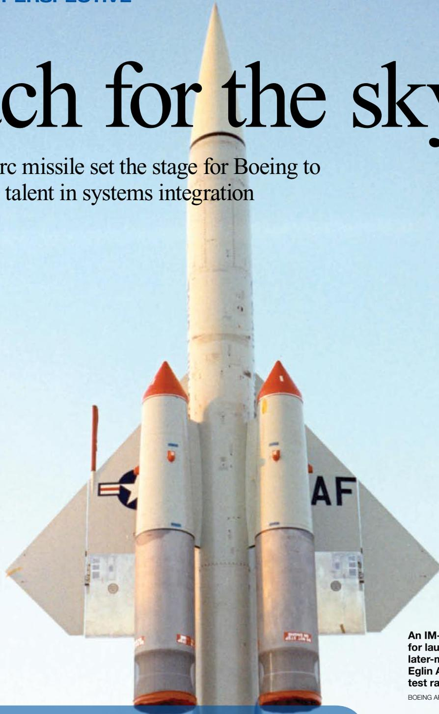
An IM-99B Bomarc is ready for launch from one of the later-model shelters at the Eglin Air Force Base, Fla., test range in 1962.
