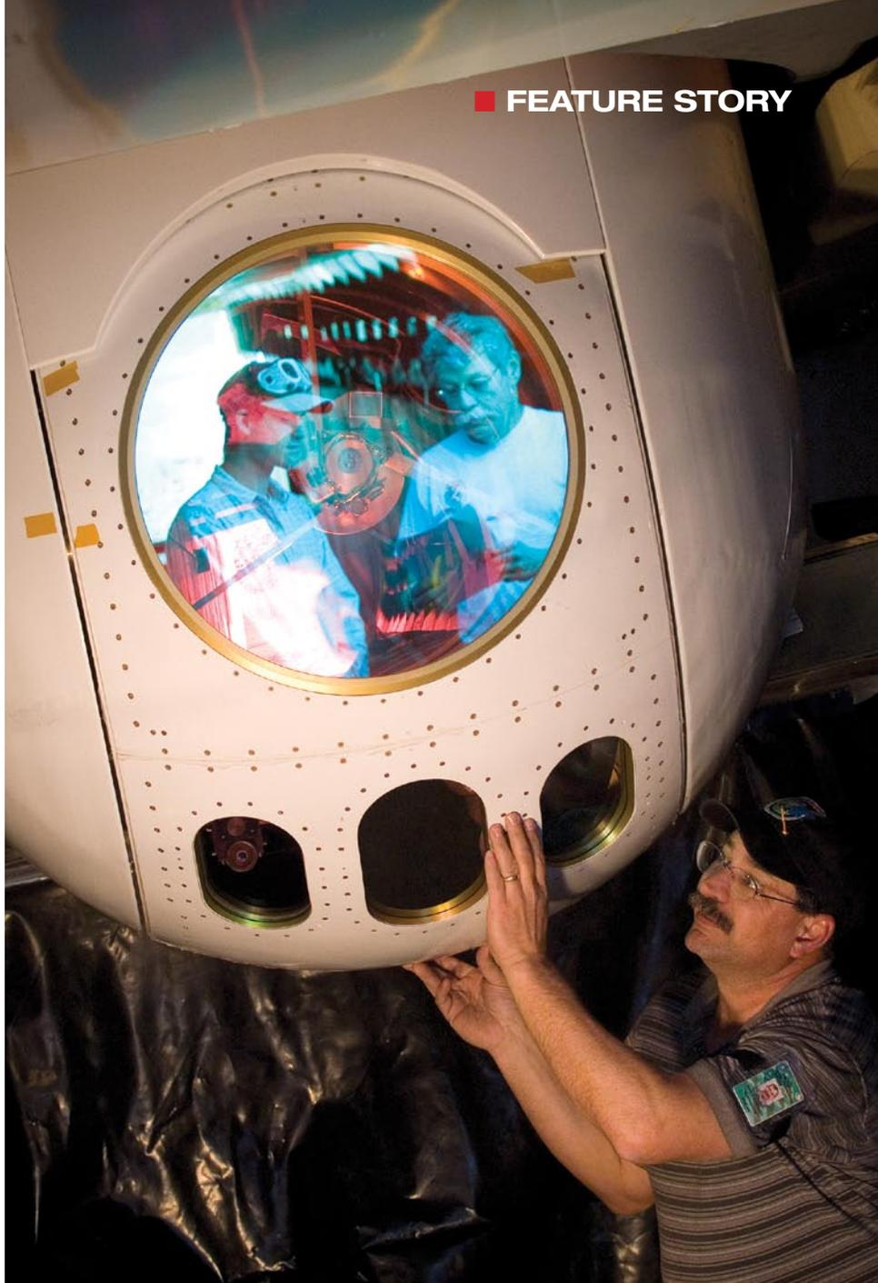
Sean Burkland, engineering technician, adjusts the Advanced Tactical Laser turret below a C-130 aircraft, as a transparent cover reflects images of Boeing-LTS mechanical engineer Jim Johnson (left) and engineering technician Stuart Penner.
