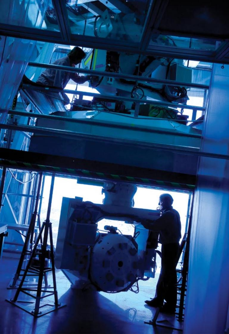
**Boeing-SVS Associate Technical Fellow Mary Jo Duncan (above) examines the transmitter telescope of the Aerospace Relay Mirror System at Kirtland Air Force Base in Albuquerque, while Bill Browning, ARMS program manager, checks the receiver telescope and its gimbal—a device that allows multidirectional movement.**
