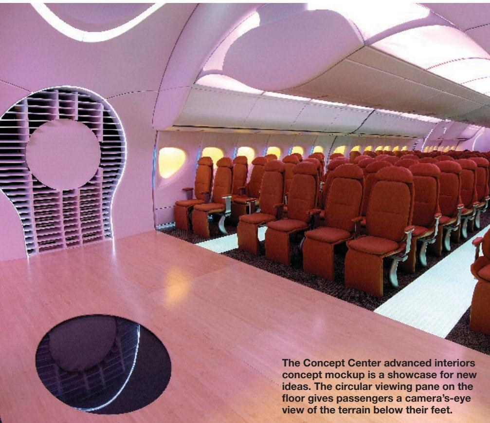
The Concept Center advanced interiors concept mockup is a showcase for new ideas. The circular viewing pane on the floor gives passengers a camera's-eye view of the terrain below their feet.
