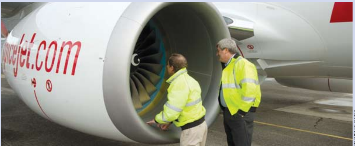
Once the test pilots have completed the necessary paperwork, they head out to the flight line to begin a series of checks outside the aircraft. Here Assistant Chief Production Test Pilot Gary Meiser (left) and Production Test Pilot Greg Guest perform a preflight inspection of a 737's engines.
