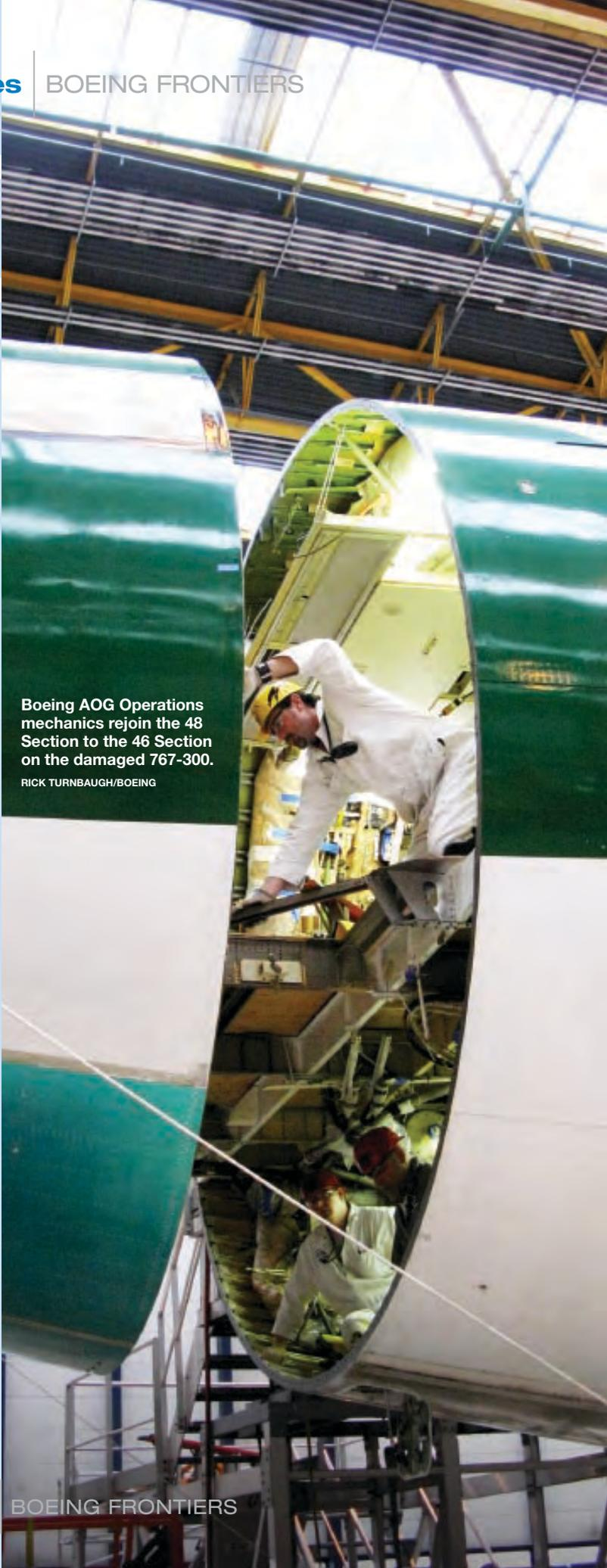
Boeing AOG Operations mechanics rejoin the 48 Section to the 46 Section on the damaged 767-300.
