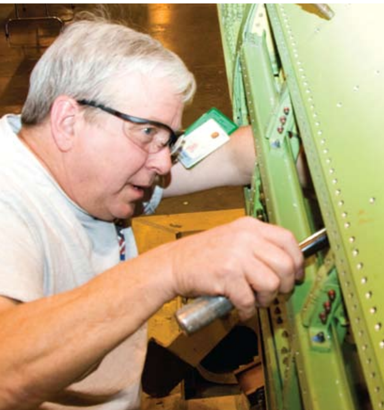
PHOTO: Jim Bryant, a modification mechanic, assembles an engine strut for a special-mission Boeing KC-135. BEVERLY NOWAK/BOEING
