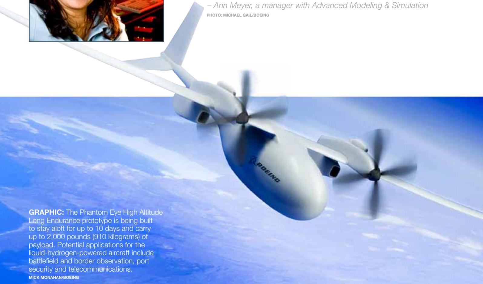
**GRAPHIC:** The Phantom Eye High Altitude Long Endurance prototype is being built to stay aloft for up to 10 days and carry up to 2,000 pounds (910 kilograms) of payload. Potential applications for the liquid-hydrogen-powered aircraft include battlefield and border observation, port security and telecommunications.
