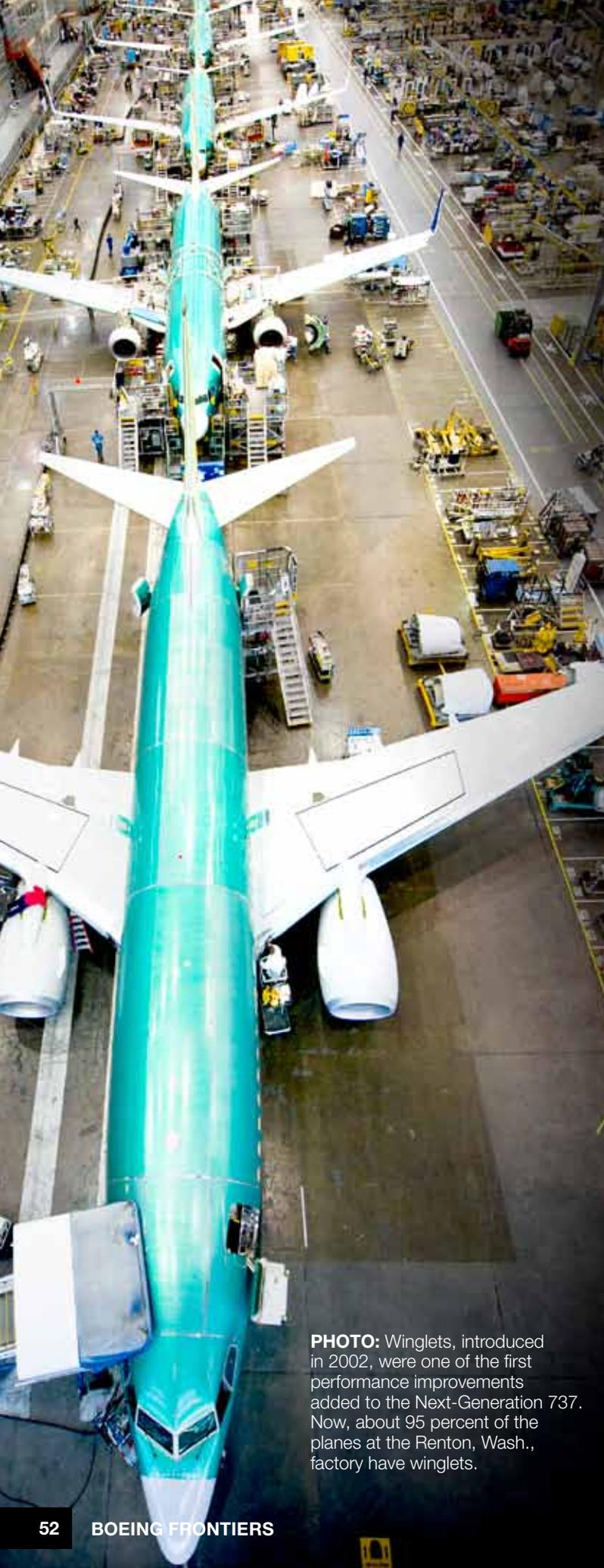
**PHOTO:** Winglets, introduced in 2002, were one of the first performance improvements added to the Next-Generation 737. Now, about 95 percent of the planes at the Renton, Wash., factory have winglets.
