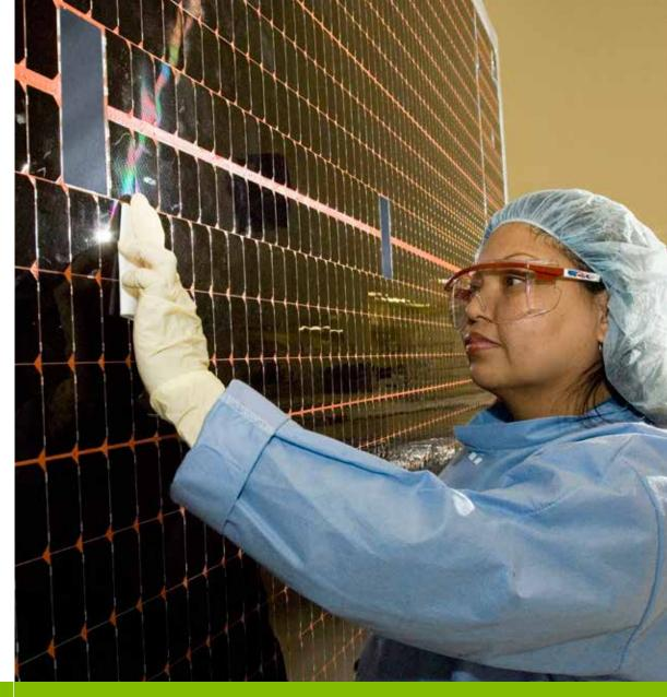
A technician at Spectrolab inspects a section of a solar panel that will eventually power a satellite. (Boeing photo) In 2013, Spectrolab set a new world record by producing a solar cell that converted 38.8 percent of solar energy into electricity, beating its previous own world record of 37 percent. The next year, Spectrolab set another record and became the first company to produce 4 million gallium arsenide-based solar cells for use in space.
