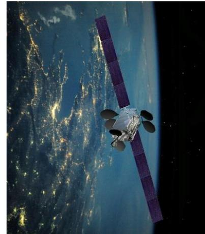
The new contract announced in May 2013 adds four more Epic<sup>NG</sup> satellites to the Intelsat fleet, starting with Intelsat 33e to be launched in 2016. The Intelsat satellites incorporate low-risk, proven technologies based on the Boeing 702HP satellite. The payload is powered by two solar wings, each with three panels (Intelsat 22 and 27) or four panels (Intelsat 21) of ultra triple-junction gallium arsenide solar cells.
