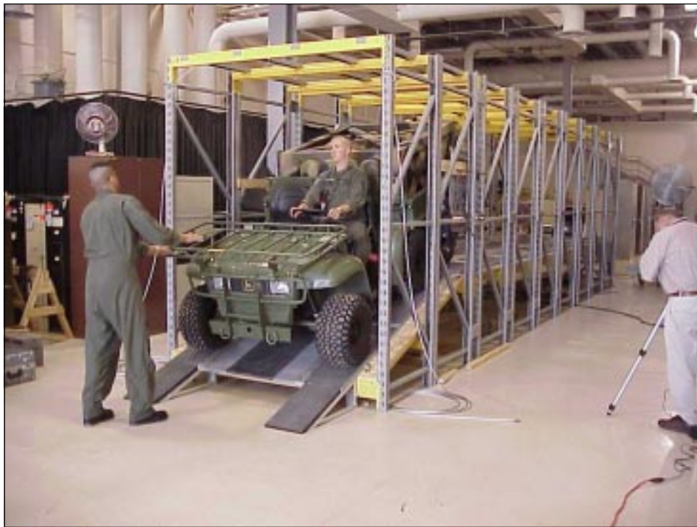
The cargo mockup lab is a dimensional replica of the cargo bay found on an MV-22 production aircraft.
