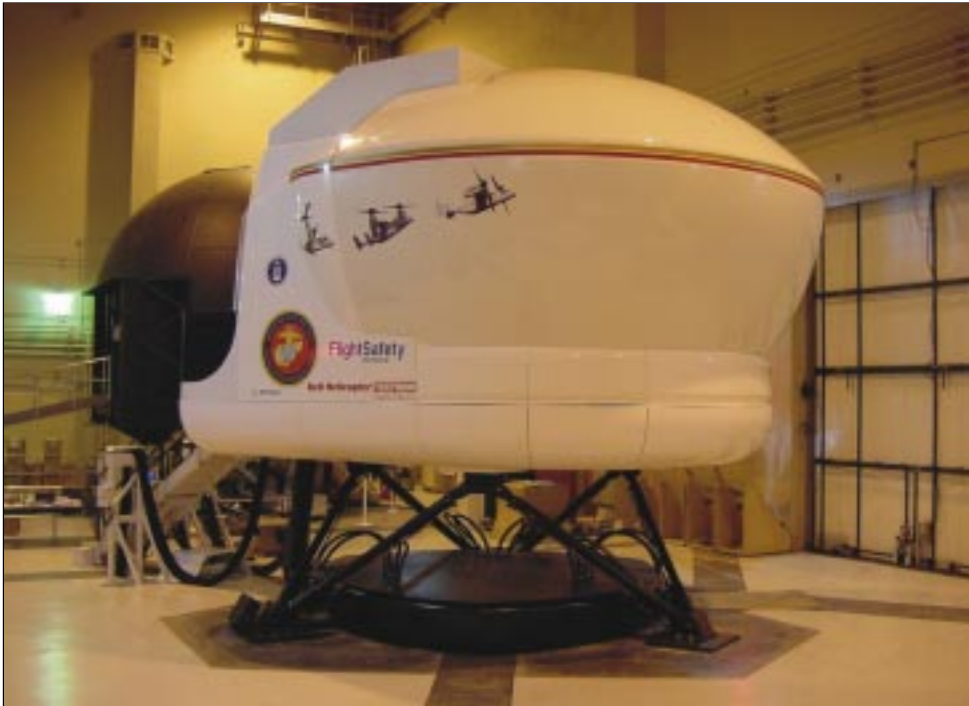
The V-22 Full Flight Simulator is the first of 32 training devices that will be delivered to the Marines, Air Force and Navy over the next 14 years. The simulator will help decrease crew and aircraft attrition.
