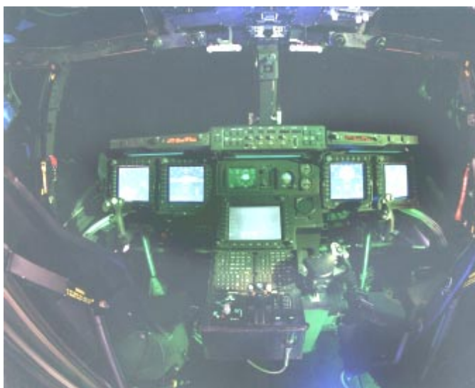
The V-22 cockpit has been modified to receive flat panel multi-function display technology, saving $500 million in procurement costs. (Dave Martin photo)
