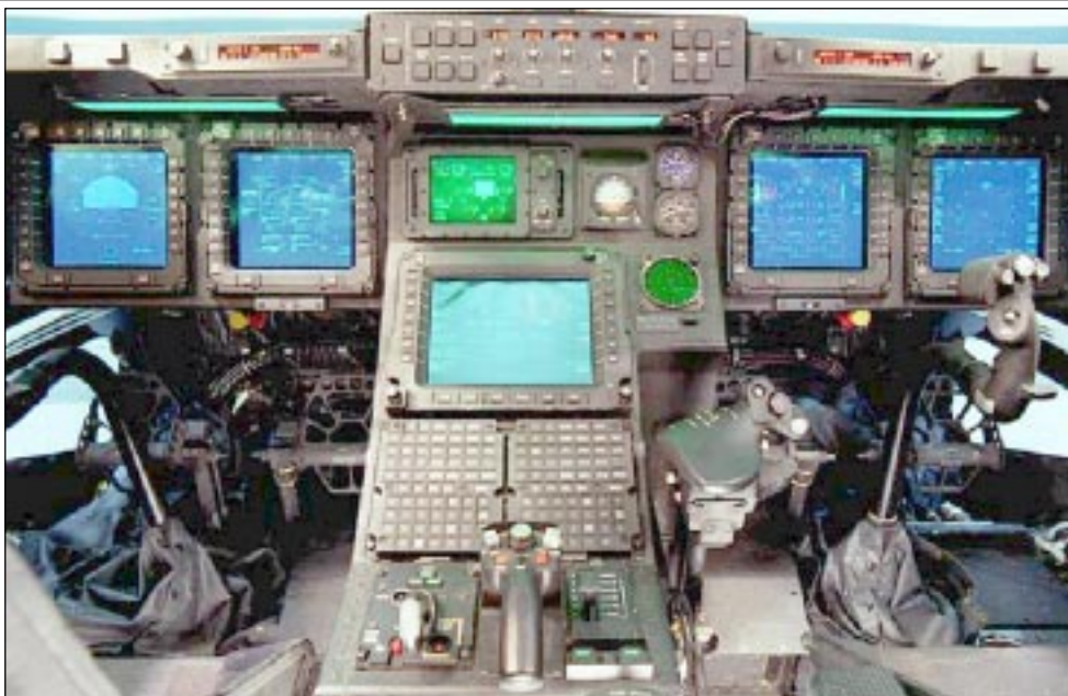
The V-22 Osprey's state-of-the-art cockpit offers completely integrated hardware and software that reduce pilot workload, and constitutes one of the most advanced cockpit designs available.
