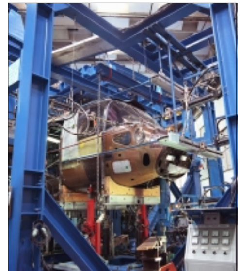
A V-22 Osprey undergoes testing of its components during the Airframe Fatigue Test Program.
