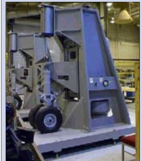
The Landing Gear Part Task Trainers, also built at Boeing Mesa, consist of two identical units constructed entirely from original components. They simulate the full mass of the aircraft on the main landing gear (15,000 pounds) by using pneumatic pressure. It was delivered in April 2002, six months ahead of schedule.
