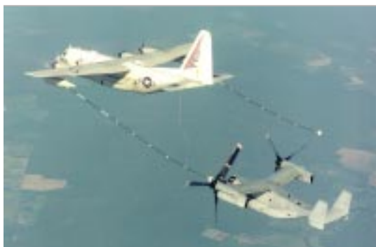
The V-22's aerial refuel capability was demonstrated during a non-stop, 2,250 naut. mile cross-country flight.
