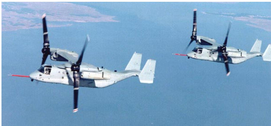
The V-22 has demonstrated 265 knots - maximum level speed; and a 25,000 foot altitude service ceiling.
