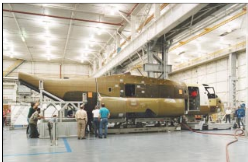
Boeing workers watch as the aft fuselage of V-22 number 11 slides into place. The forward section, containing the cockpit and avionics racks, had been attached just moments before. The total time required to join the three sections was twenty minutes.
