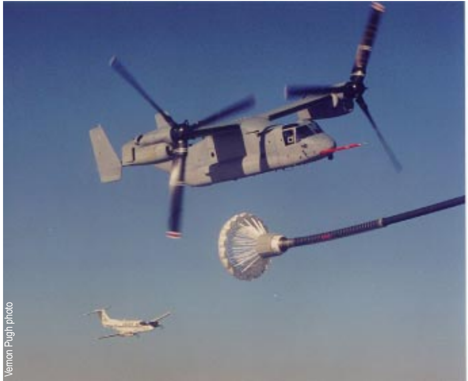
During simulated aerial refueling flights, the V-22 holds its position near the refueling drogue behind a KC-130 tanker (not shown). The King Air chase plane is in the background.
